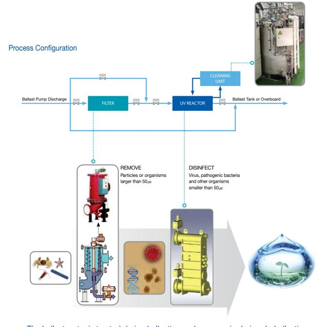
The ballast water is treated during ballasting and once again during de-ballasting.
