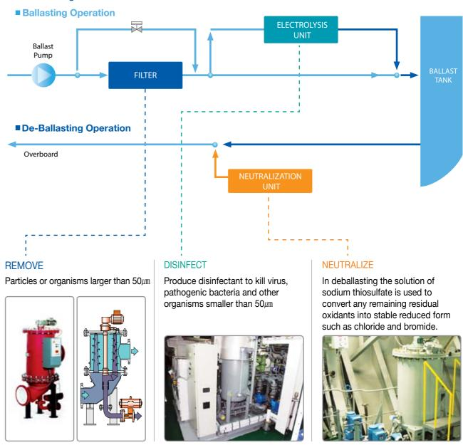
In deballasting operation, the system needs to be neutralized prior to the discharge with neutralization agent to avoid environmental damage of the sea water.
