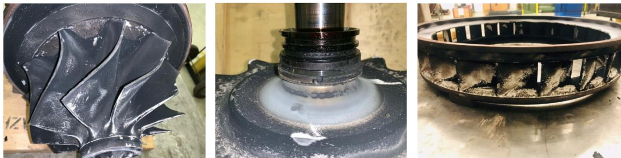
Figure 1. White deposit on turbocharger components
