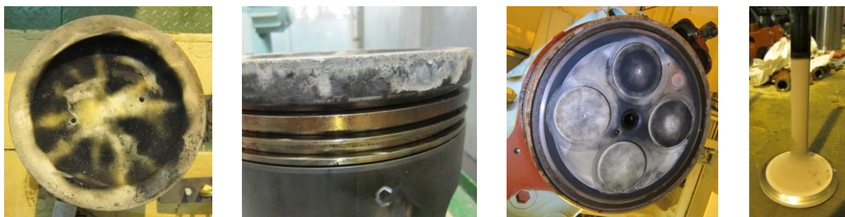
Figure 2. White deposit on combustion chamber components
