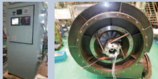
Rotor with magnets and a stator winding installed on the MET83SE turbocharger
