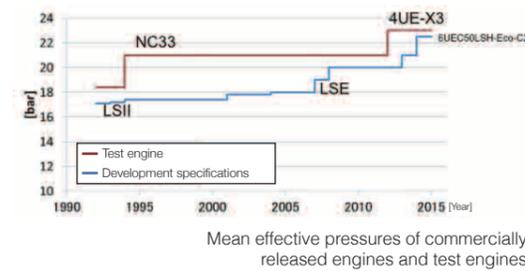
From around 2006, MHI began releasing the UEC-LSE series, which boasted even higher fuel efficiency and reliability, with the good Sevie records of the aforementioned LSII series. The roll-out pace of electronically-controlled engines in the series also increased aggressively in response to needs for greater fuel efficiency and conformity to NOx emission reduction requirements.
