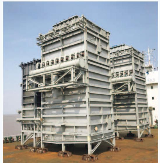
DIA-SOx® R-type marine SOx scrubber (flue gas desulfurization system)
