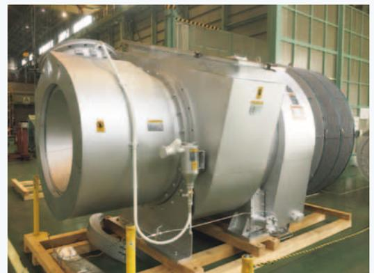
MET Turbocharger mounted on a 12X92DF engine
