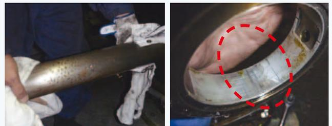
Case in which the journal bearing broke while the rotor was being pulled out because of corrosion and scratches on the surface of the rotor guide tube
