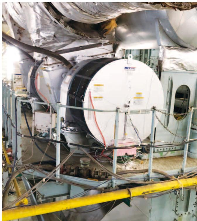
MET60MBII mounted on the test engine (6X72DF)
