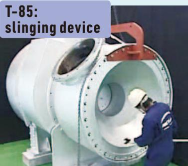
Attach slinging device(T-85) to gas inlet casing
