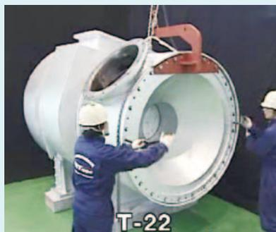
Screw 2 lifting screws(T-22) & lift slowly using a cable with chain block.
