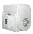
Horizontal, foot mounted, squirrel cage type rotor, IM1001, IP-44 IC611, with top mounted air cooled air cooler, self air circulation,
