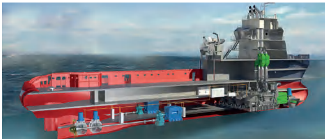
EPROX propulsion solution on anchor handling tug supply vessel
