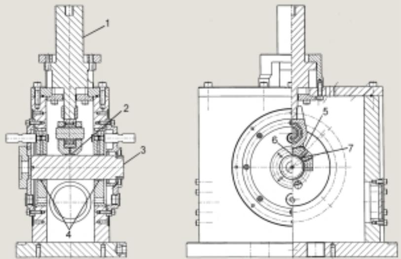
Figure 10: Section drawing of the small bearing test bench
