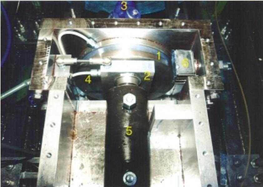
Figure 15: Test bench for sliding block experiments
