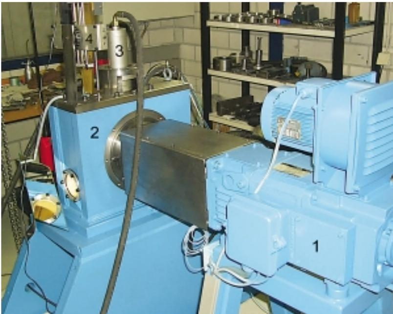
Figure 8: Small bearing test bench
