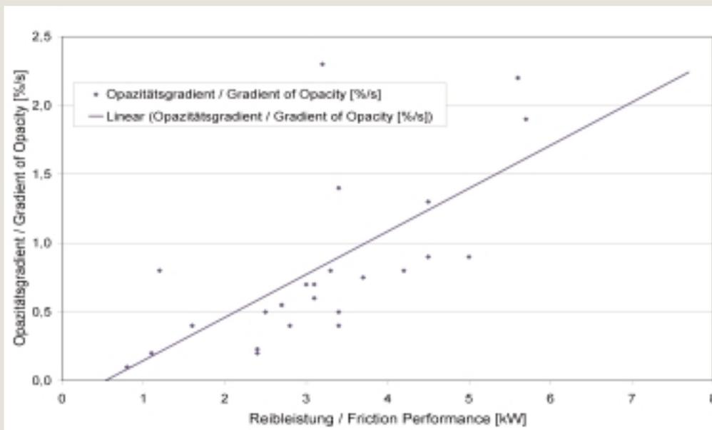
Figure 12: Gradient of opacity vs. friction performance for measurements on the small test bench
