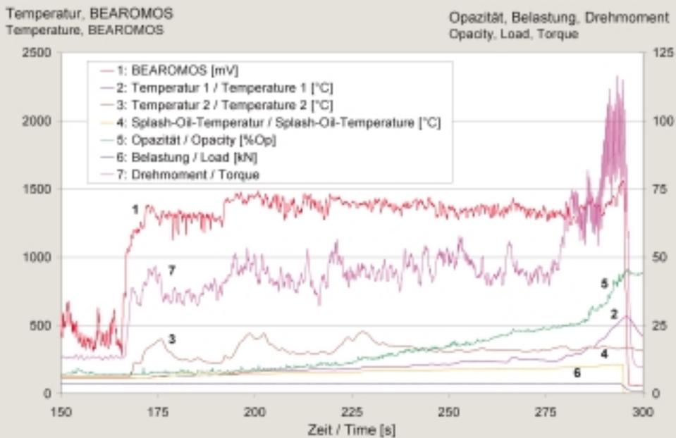
Figure 13: Measurement on the large test bench under static loading
