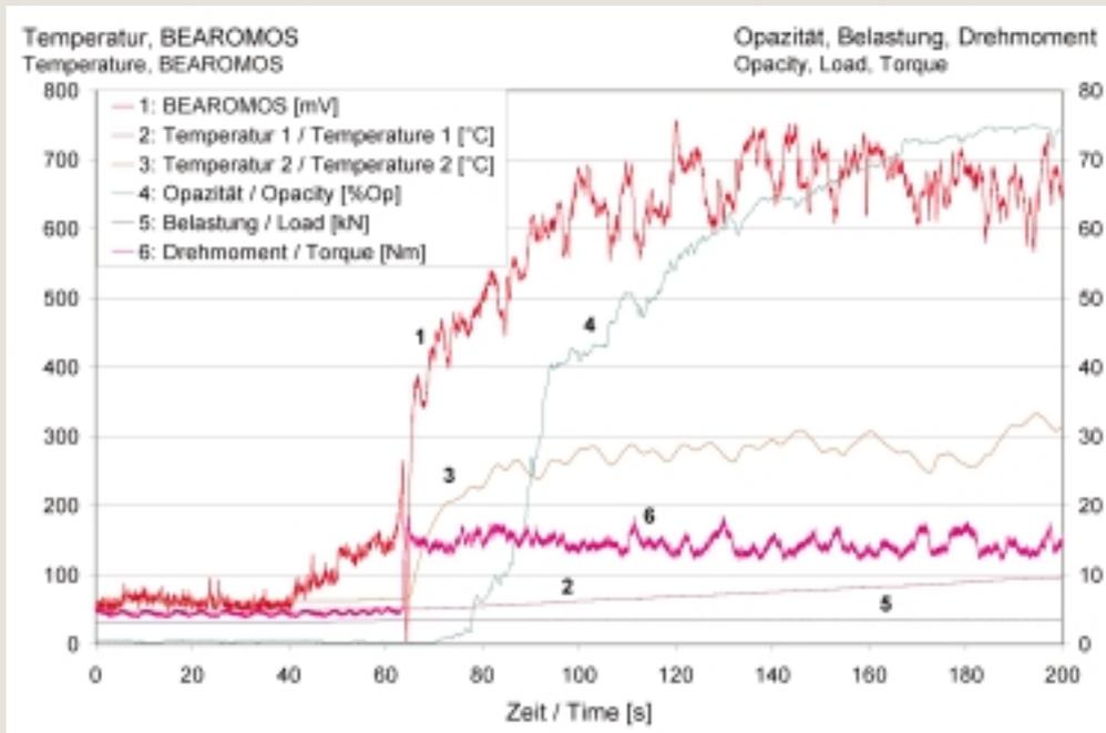
Figure 11: Measurement on the small test bench under static loading with a bronze-half plain-bearing shell loading force 3,7 kN, average bearing pressure 6,3 N/mm<sup>2</sup>, Oil inlet temperature 40° C
