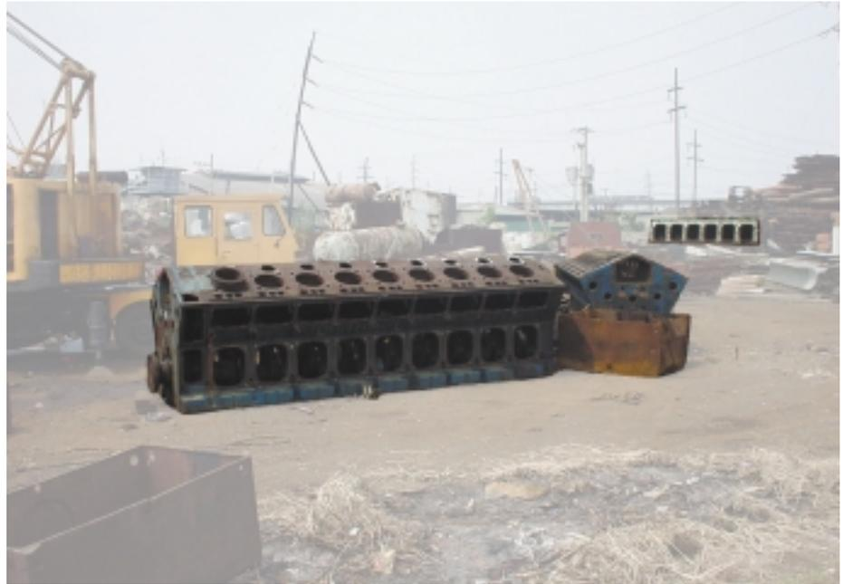
Figure 1: A crankcase explosion can destroy an engine down to scrap
