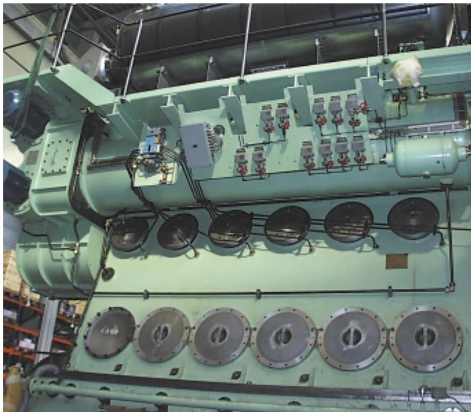
Figure 3: Oil mist detector installed on a crosshead two-stroke engine. Power output 9 MW (output up to 70 MW per unit can be realized)
