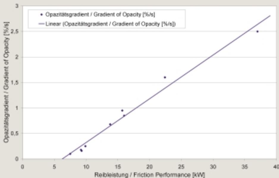
Figure 14: Gradient of opacity vs. friction performance for the measurements on the large test bench
