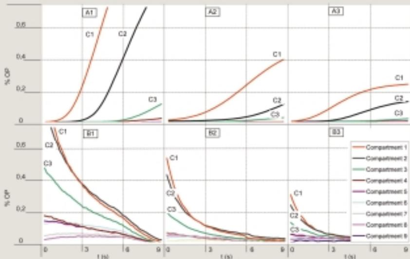
Figure 16: Oil mist induction A, Oil mist dissipation B for the consecutive compartments 1 to 9 of the medium speed engine (Opacity: % OP)
