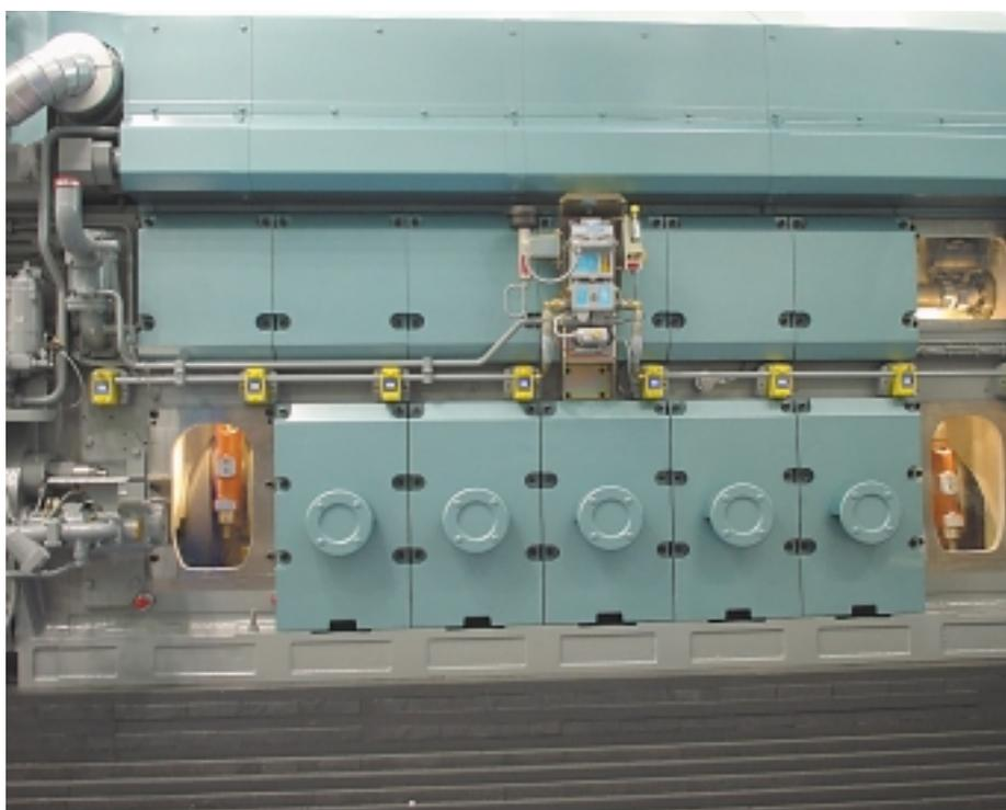
Figure 4: Oil mist detector installed on a four-stroke diesel engine, 2,4 MW, up to 50 MW per unit can be realized
