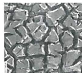
Figure 5. Electrode Surface after Coating
