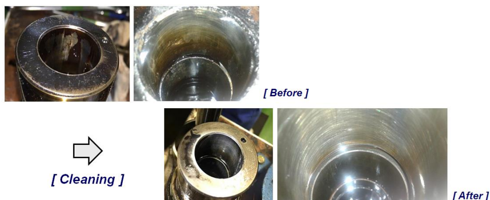
Fig.2 Before and after condition of STUCK barrel of fuel injection pump
