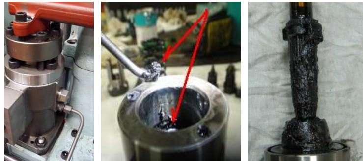
Fig.3 Drain line of fuel injection pump and contaminated condition by sludge
