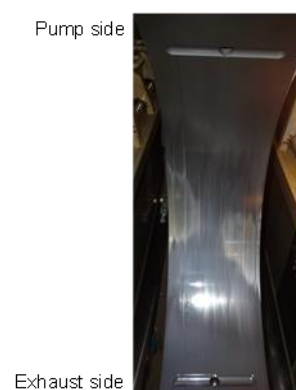
Figure 15. UEC50LSH-Eco-C2 Crank pin bearing metal condition (13,663 running hours)
