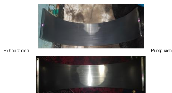
Figure 13. UEC50LSH-Eco-C2 Main bearing metal condition (13,663 running hours)
