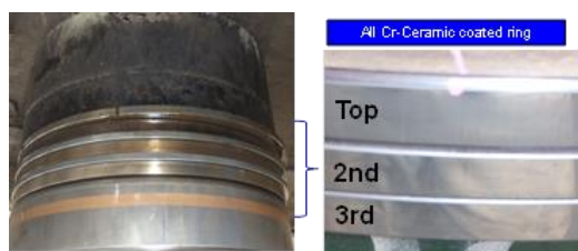
Figure 11. UEC50LSH-Eco-C2 Piston rings condition (13,663 running hours)
