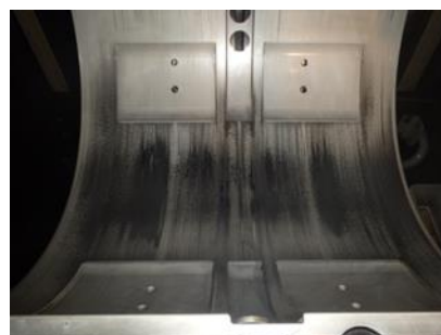
Figure 14. UEC50LSH-Eco-C2 Crosshead pin bearing metal condition (13,663 running hours)
