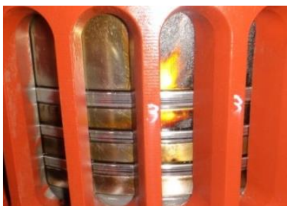
Figure 28. piston ring condition (approx.80 running hours)
