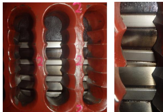
Figure 14. Inspection result of piston rings
