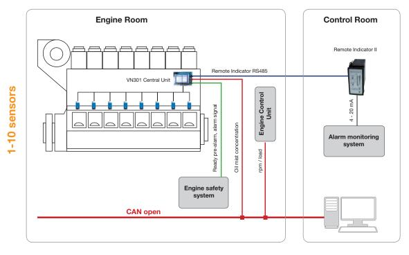
sensors ensure that the crankcase is monitored.
