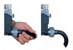
The engine wall screw fitting with its flexible intake funnel is mounted from the outside. Its form prevents splash oil from being drawn in and a false alarm being triggered. We can offer you a suitable engine wall screw fitting to match the engine wall thickness.
