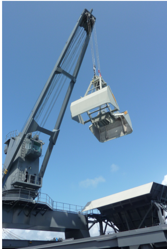
Gantry travelling type jib crane.
